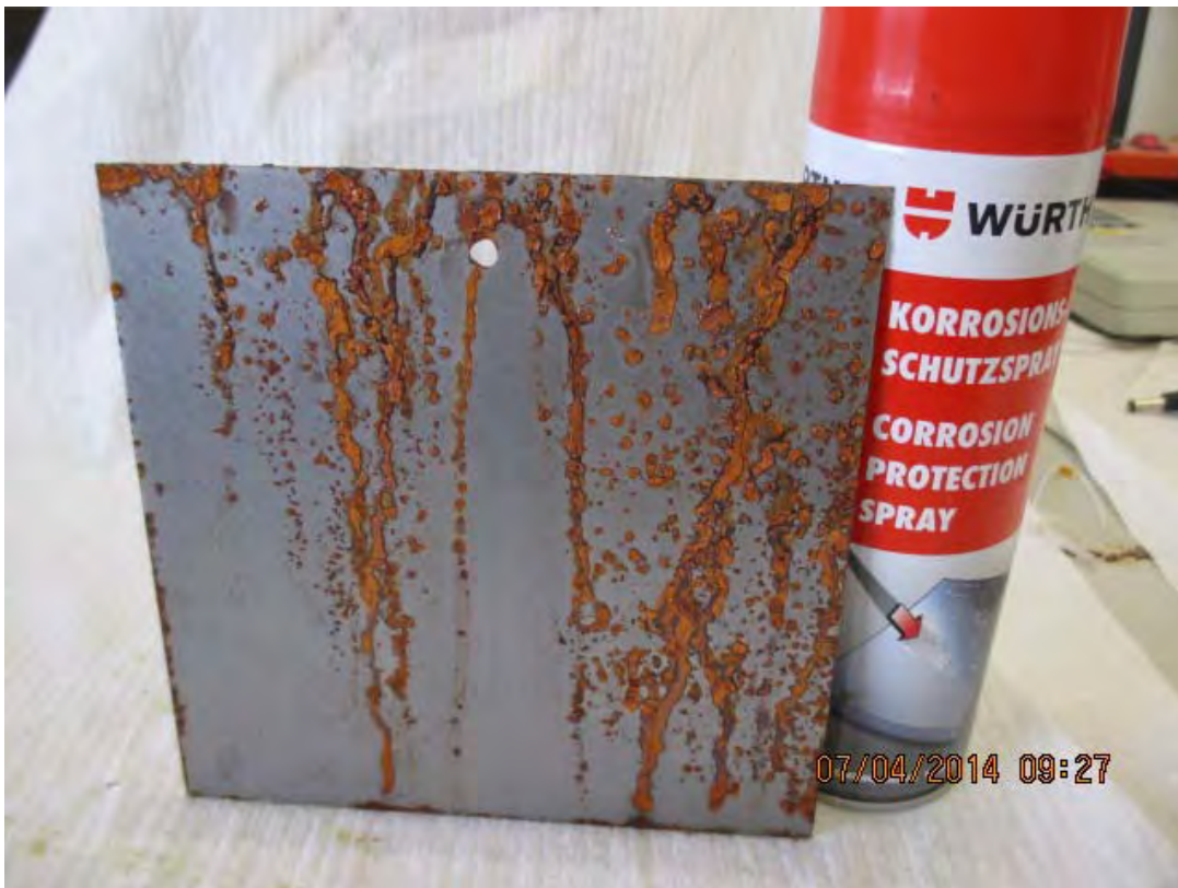
Pic. 21 Metal plate #4 after 96h salt fog exposure
