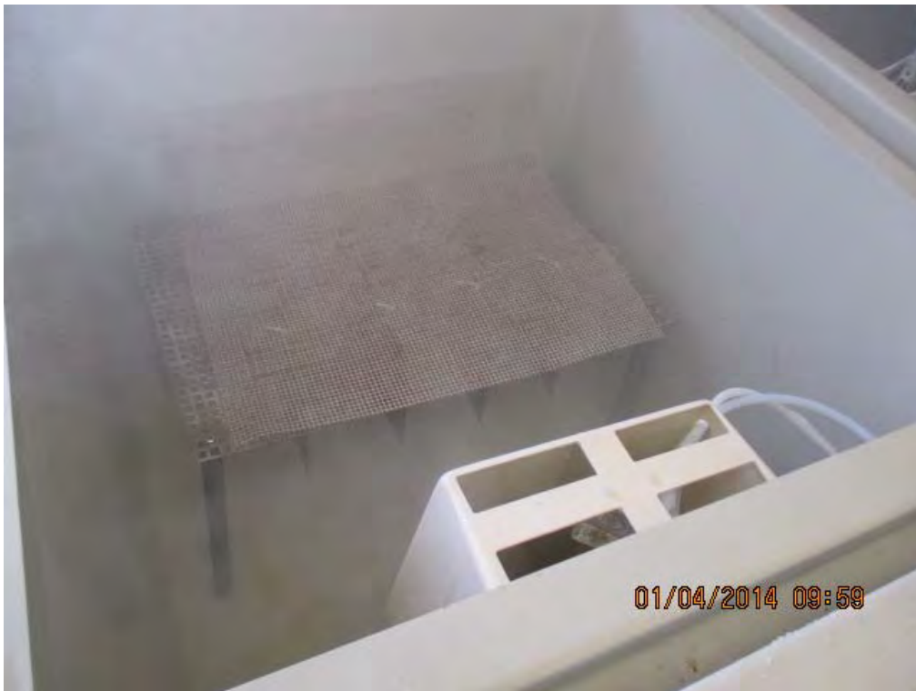
Pic. 5 EUTs in the salt spray chamber
