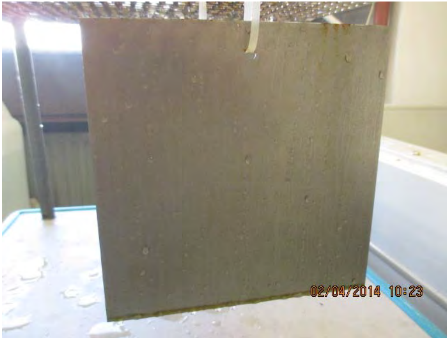
Pic. 6 Metal plate #1 after 24h salt fog exposure
