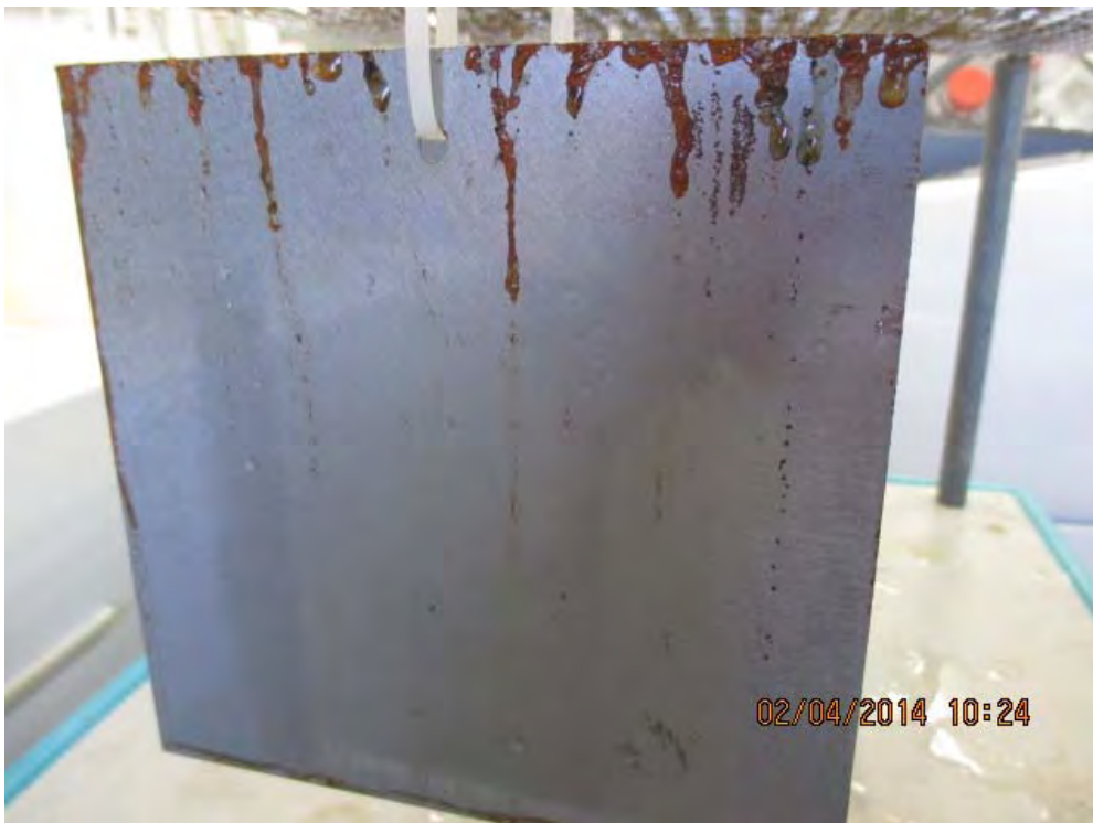
Pic. 9 Metal plate #4 after 24h salt fog exposure
