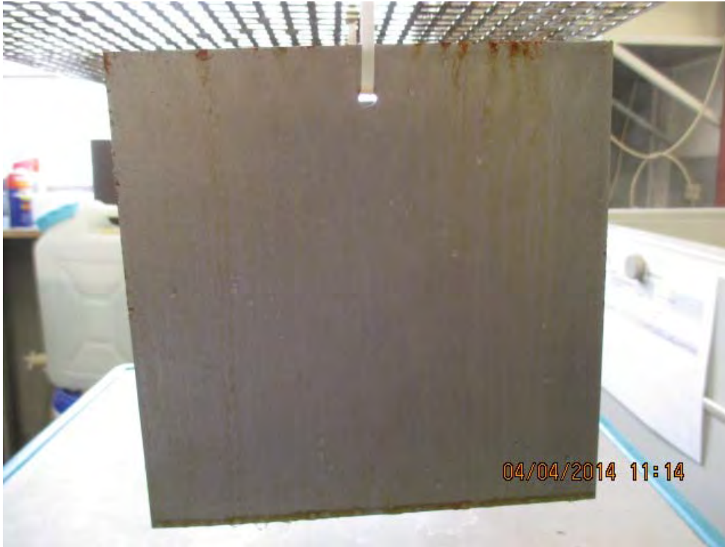
Pic. 14 Metal plate #1 after 72h salt fog exposure
