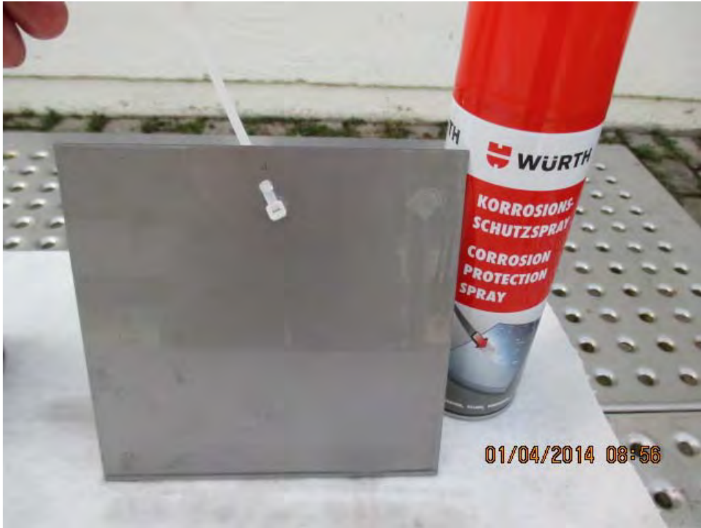
Pic. 4 Metal plate #4 coated with Würth Corrosion Protection Spray
