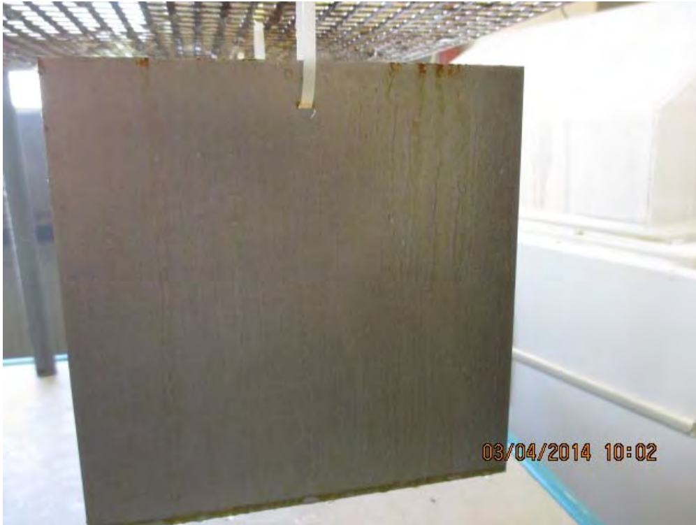
Pic. 10 Metal plate #1 after 48h salt fog exposure
