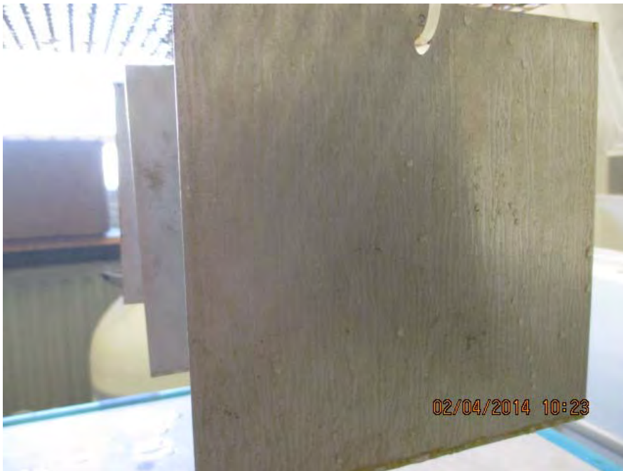
Pic. 7 Metal plate #2 after 24h salt fog exposure
