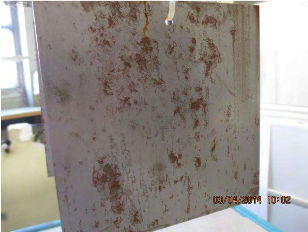
Pic. 12 Metal plate #3 after 48h salt fog exposure
