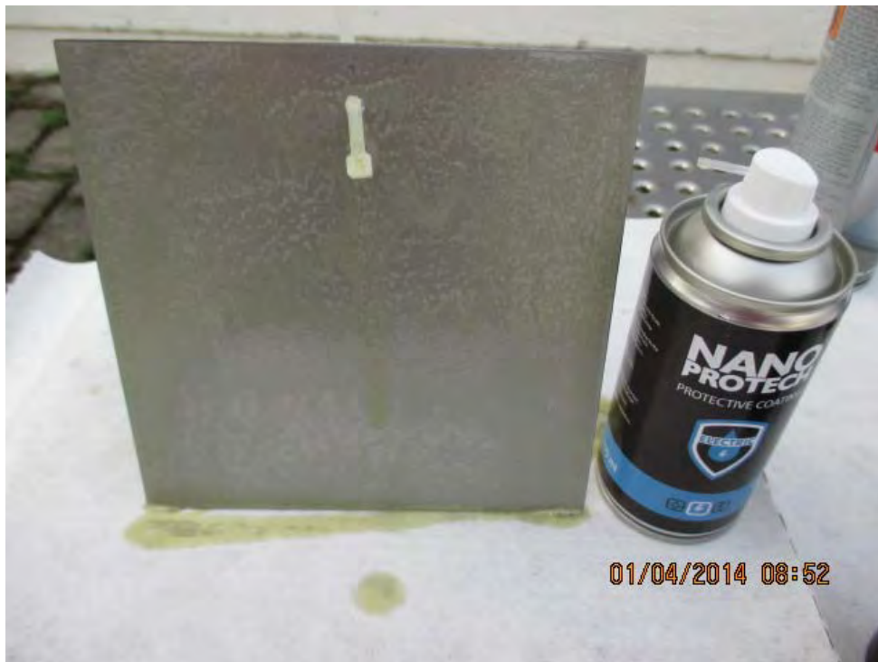
Pic. 1 Metal plate #1 coated with Nano Protech Electric
