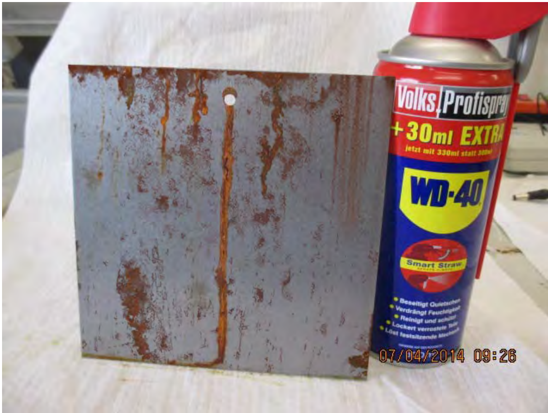
Pic. 20 Metal plate #3 after 96h salt fog exposure
