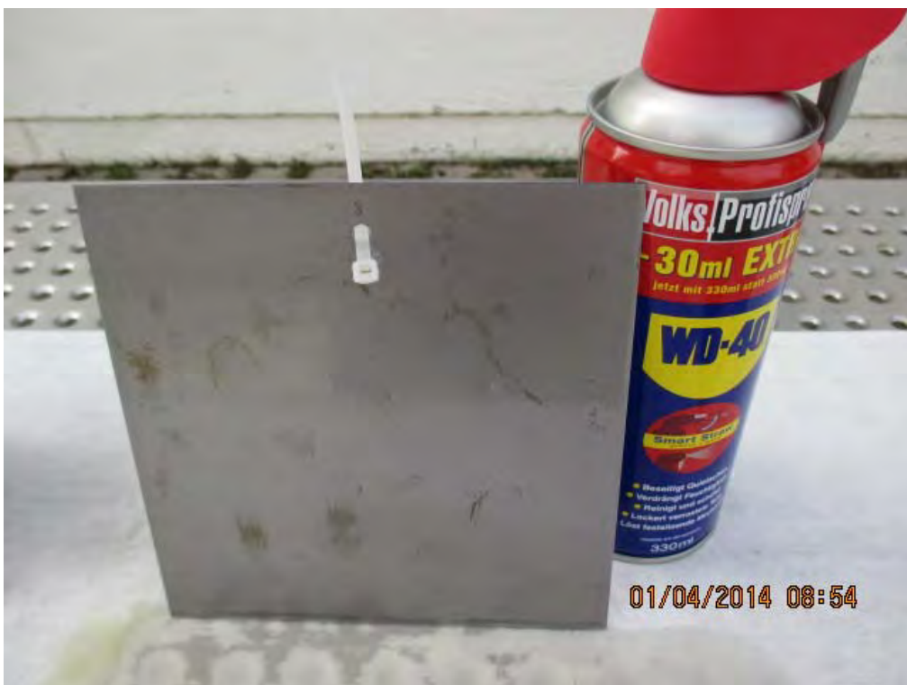
Pic. 3 Metal plate #3 coated with Oil Spray WD40
