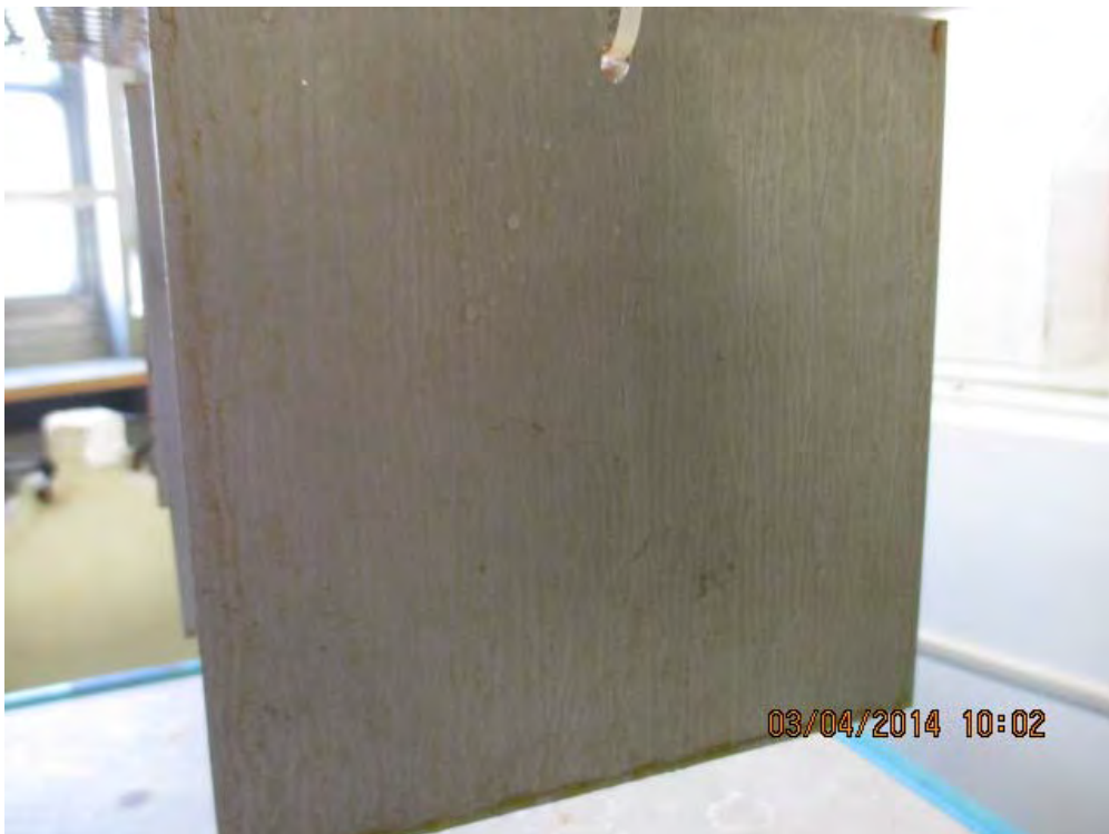
Pic. 11 Metal plate #2 after 48h salt fog exposure
