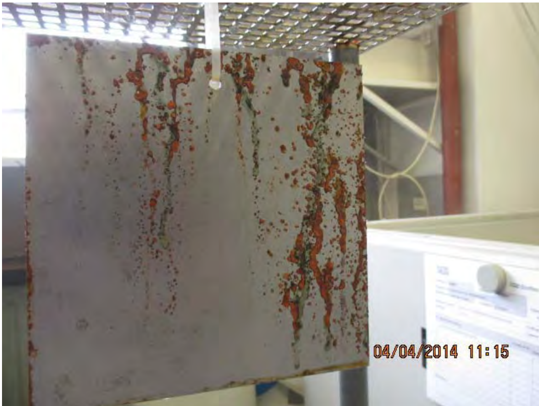
Pic. 17 Metal plate #4 after 72h salt fog exposure
