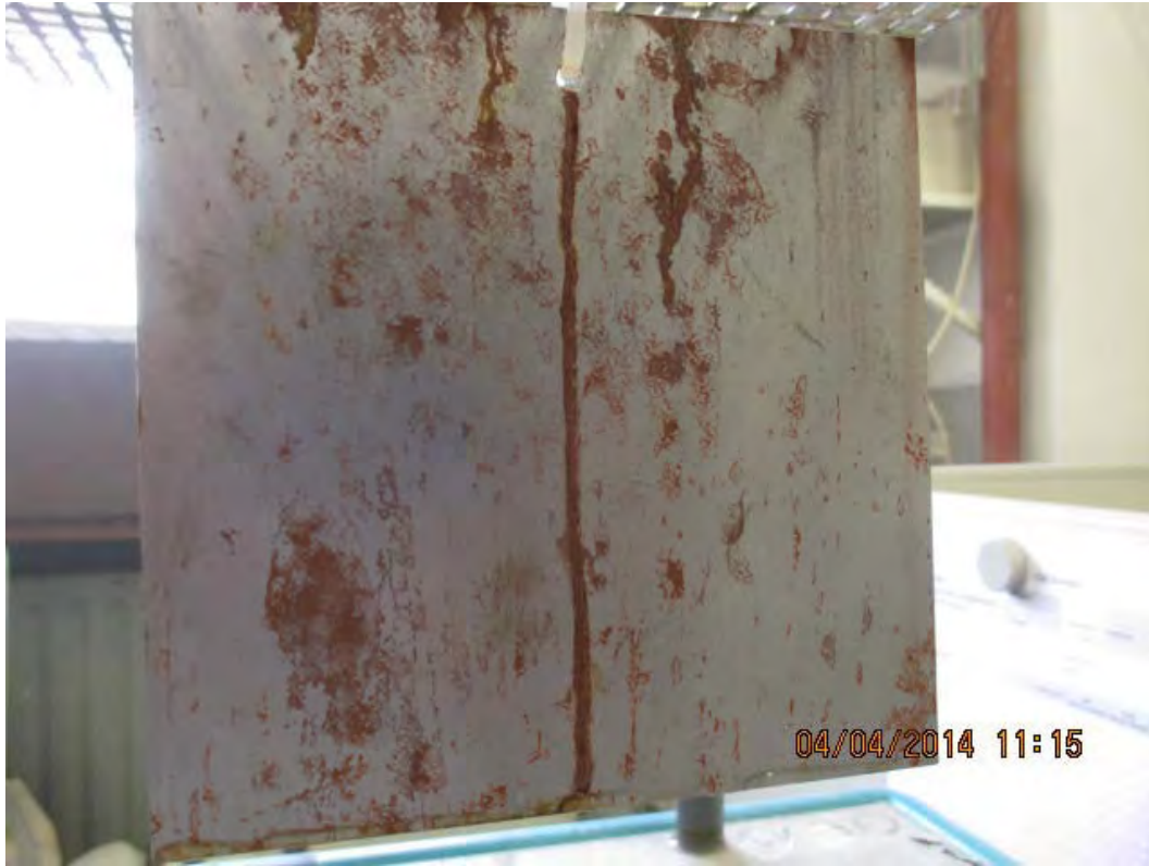
Pic. 16 Metal plate #3 after 72h salt fog exposure
