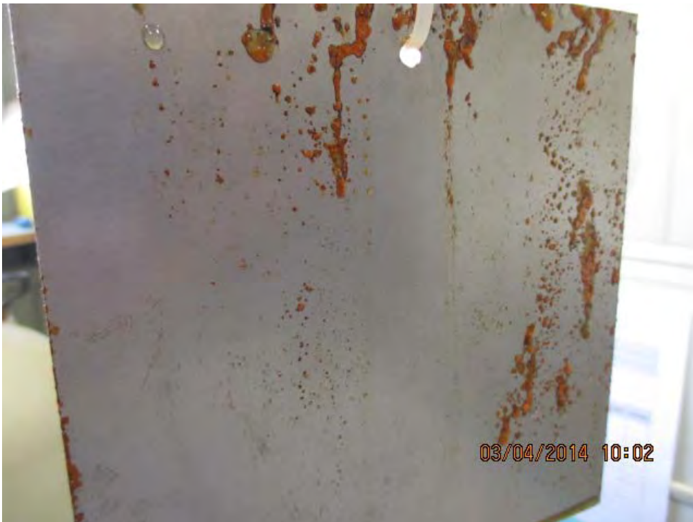
Pic. 13 Metal plate #4 after 48h salt fog exposure
