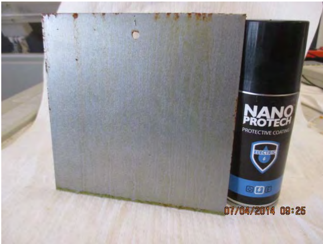
Pic. 18 Metal plate #1 after 96h salt fog exposure
