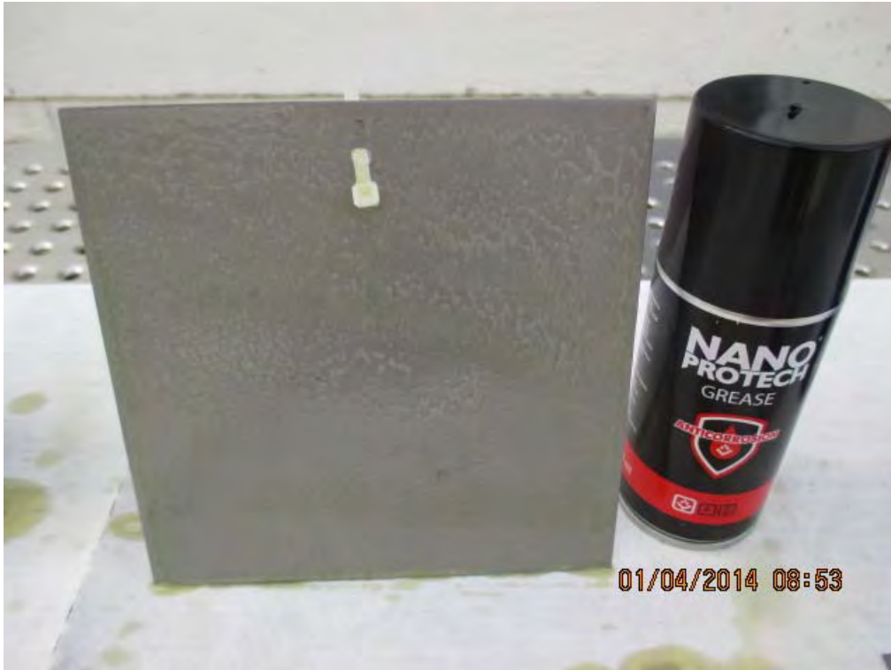
Pic. 2 Metal plate #2 coated with Nano Protech Grease Anti Corrosion
